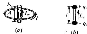
Figure 6-4 (a) Relation of small loop of area A to short magnetic dipole of length l . (b) Short magnetic dipole.
