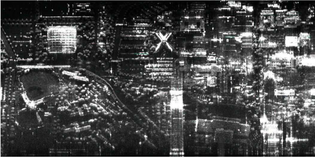
Figure 2.13: A YINSAR image of BYU campus with motion compensation applied.
