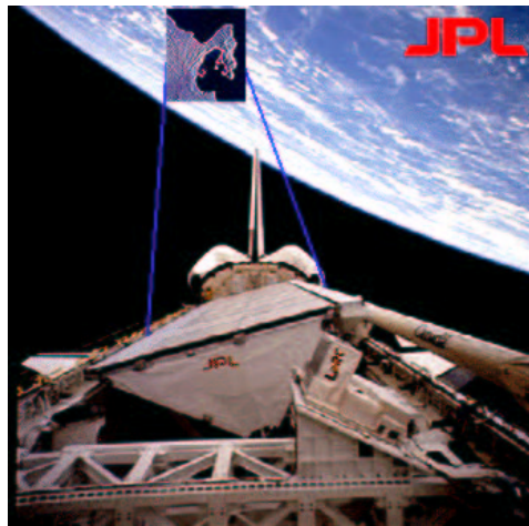
Figure 2.2: SIR-C/X-SAR aboard the space shuttle at an orbit altitude of 225 km. Courtesy of NASA/JPL.
