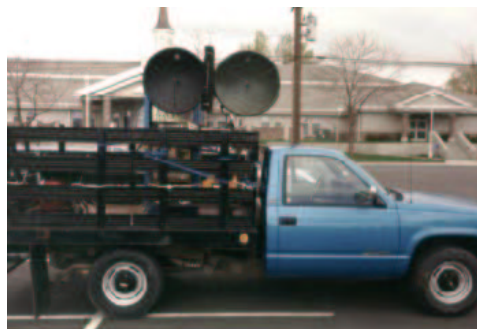
Figure 2.9: Truck platform used to deploy BYUSAR
