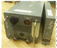
**RT-1159** - The receiver/transmitter demodulates TACAN transmissions and also transmits distance interrogations. The R/T gives 3 major outputs: **relative** bearing, range and beacon audio.
