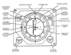
Bearing - Magnetic bearing to your station is indicated by the BEARING POINTER.
