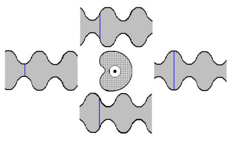
So basically, the aircraft determines its bearing from the station by looking at the waveform of the signal and where the main reference burst is pulse encoded. To provide more accurate bearing information, TACAN uses the same principle again to calculate fine bearing. Yet another rotating element with **9** reflectors produces even more amplitude variations. Again, there is a reference point for the variable amplitude variations. This comes in the form of **9** auxillary reference bursts:
