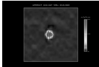
Figure 12: Radio map of the same region of sky plotted in Figure 14, showing that the unwanted emissions from the geostationary broadcasting satellite are easily detected in the frequency band 1660 - 1670 MHz that is allocated to the Radio Astronomy Service on a primary basis, shared with active services. Measurements were made with the Effelsberg 100-m antenna (Klaus Ruf, private communication).
