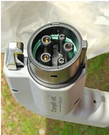
SAE J1772-2009 electric vehicle connector.
