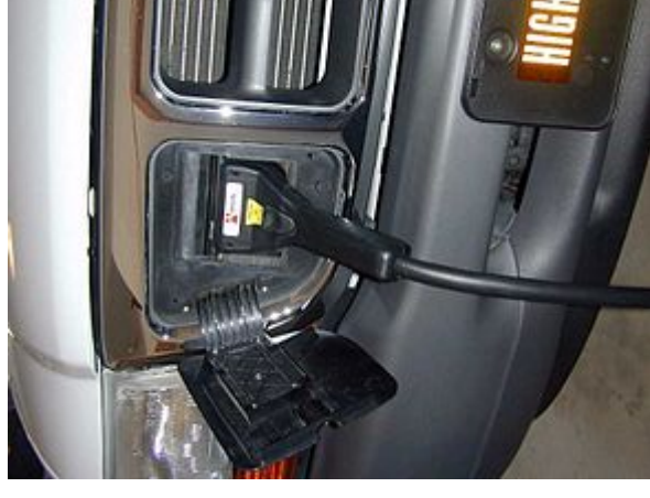
The older Avcon connector, featured here on a Ford Ranger EV
