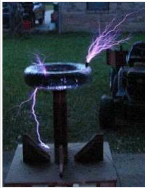
A small, later-type Tesla coil in operation: The output is giving 43-cm sparks. The diameter of the secondary is 8 cm. The power source is a 10 000 V, 60 Hz current-limited supply.
