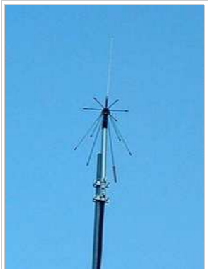
Mounted discone antenna designed for VHF and UHF coverage.
