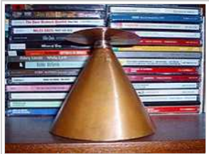
Discone made of solid copper sheets, theoretically covering 700MHz to 2GHz.
