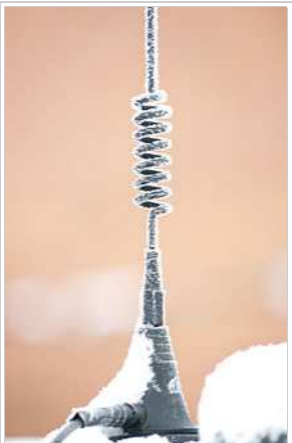
A loading coil in a small cell phone antenna on a car roof.
