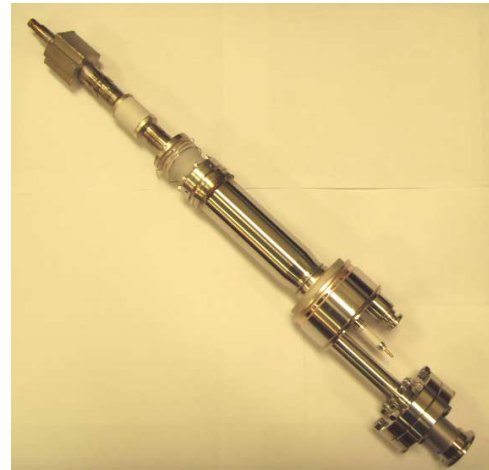
Figure 5. Vacuum-sealed W-band backward-wave oscillator.
