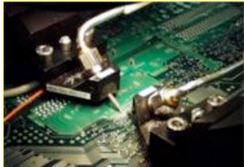
Probes Contact Directly on PWB
