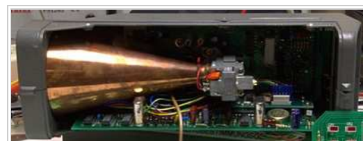
Disassembled radar speed gun. The grey assembly attached to the end of the copper-colored horn antenna is the Gunn diode oscillator which generates the microwaves.
