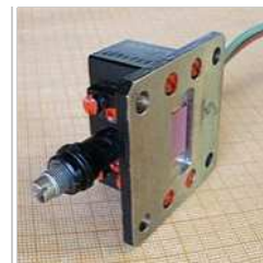
Russian Gunn diode oscillator. The diode is mounted inside the cavity ( metal box ), which functions as a resonator to determine the frequency. The negative resistance of the diode excites microwave oscillations in the cavity which radiate out the hole into a waveguide ( not shown ). The frequency can be adjusted by changing the size of the cavity using the thumbscrew.
