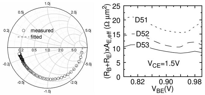
Fig. 4. Measured  $s_{11}$  at  $V_{BE}=0.92\text{V}$  from 1 to 110GHz and circle fit plotted in a Smith chart for a 8-emitter device prepared in D53 (left).  $V_{BE}$  dependence of  $R_B+R_E$  extracted from  $s_{11}$  circle fit for the HBT generations D51-D53 (right).
