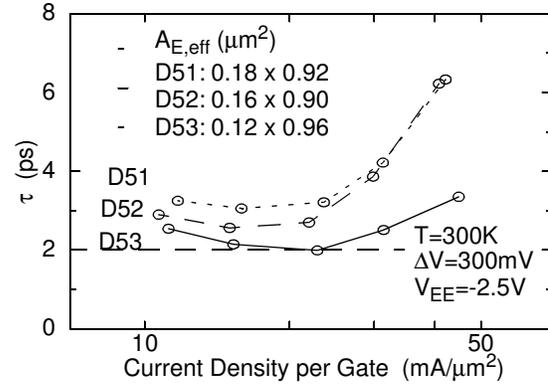
Fig. 8. CML ring oscillator gate delay  $\tau$  vs. current per gate normalized to  $A_{E,eff}$  for oscillators consisting of 53 stages with single emitter HBTs fabricated in D51-D53. Measured at  $V_{EE}=-2.5V$ ,  $\Delta V=300mV$  and  $T=300K$ .
