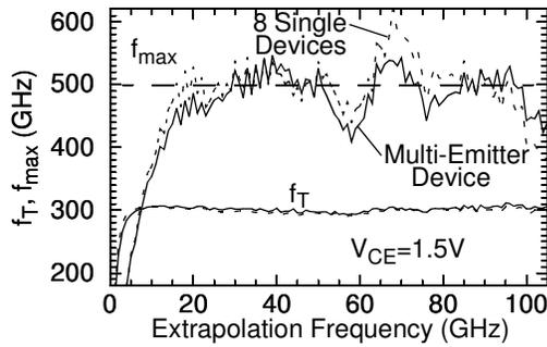
Fig. 3. Transit frequency  $f_T$  and maximum oscillation frequency  $f_{max}$  extrapolated from various frequency points with -20dB per frequency decade measured for 8 single emitter devices in parallel and a multi-emitter HBT with 8 emitters. Total effective emitter area for both is  $8 \times (0.12 \times 0.96) \mu\text{m}^2$ .  $T=300\text{K}$ .
