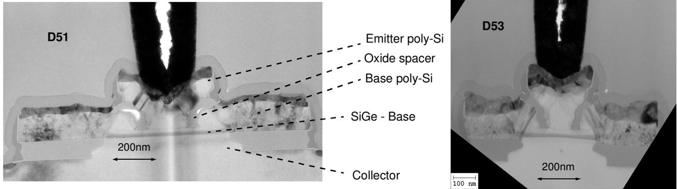
Fig. 2. TEM cross sections of the 1<sup>st</sup> (D51) and the 3<sup>rd</sup> (D53) HBT generation.
