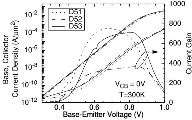
Fig. 5. Gummel plots of 8-emitter devices normalized to the effective emitter area  $A_{E,eff}$  (see Table 3) for the HBT generations D51, D52, and D53.
