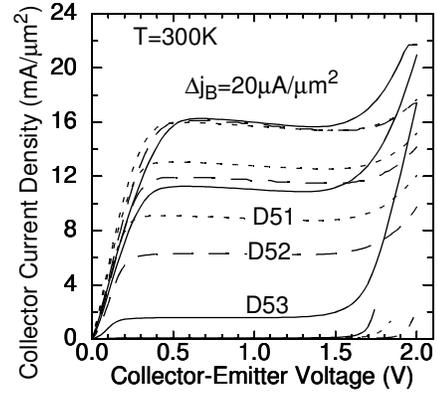
Fig. 6. Output characteristics of 8-emitter devices normalized to the effective emitter area  $A_{E,eff}$  (see Table 3) for the HBT generations D51 (dotted), D52 (dashed), and D53 (solid).
