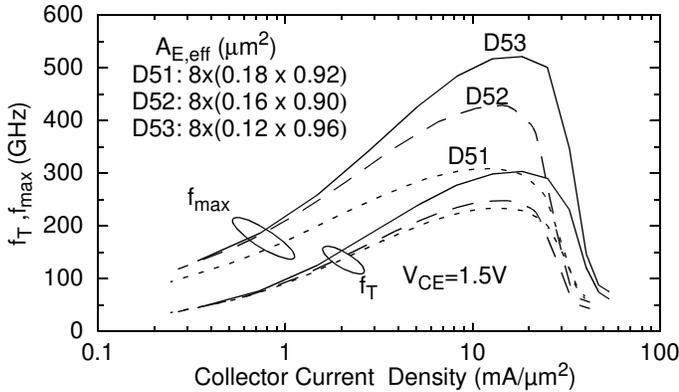
Fig. 7. Transit frequency  $f_T$  and maximum oscillation frequency  $f_{max}$  vs. collector current normalized to  $A_{E,eff}$  for the HBT generations D51-D53. Deembedded small-signal current gain  $h_{21}$  and unilateral gain  $U$  vs. frequency were used for extrapolation of  $f_T$  and  $f_{max}$  at 40GHz with -20dB per frequency decade at  $V_{CE}=1.5V$ ,  $T=300K$ .
