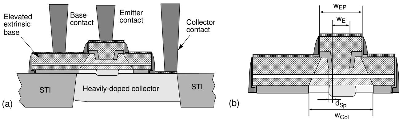
Fig. 1. Schematic cross section of the HBT under investigation (a) with key dimensions modified from generation to generation (b).
