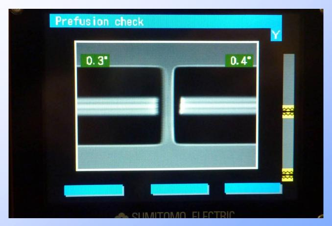
T-39 collapses the voids so it can see the core
