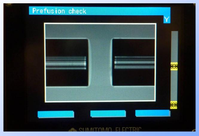
Initially the core image is shielded by the cladding voids
