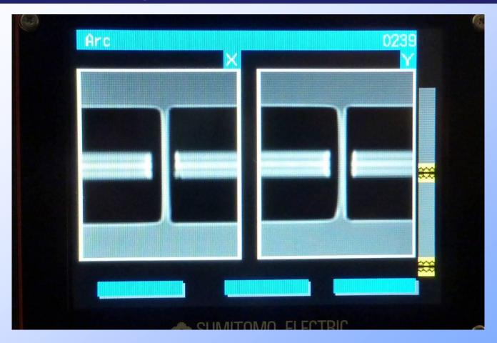
T-39 collapses the voids to image the core of the CasaLight
