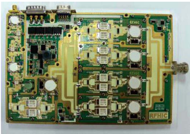
Fig. 40. Practical implementation of 1-kW S -band GaN HEMT PA [59].
