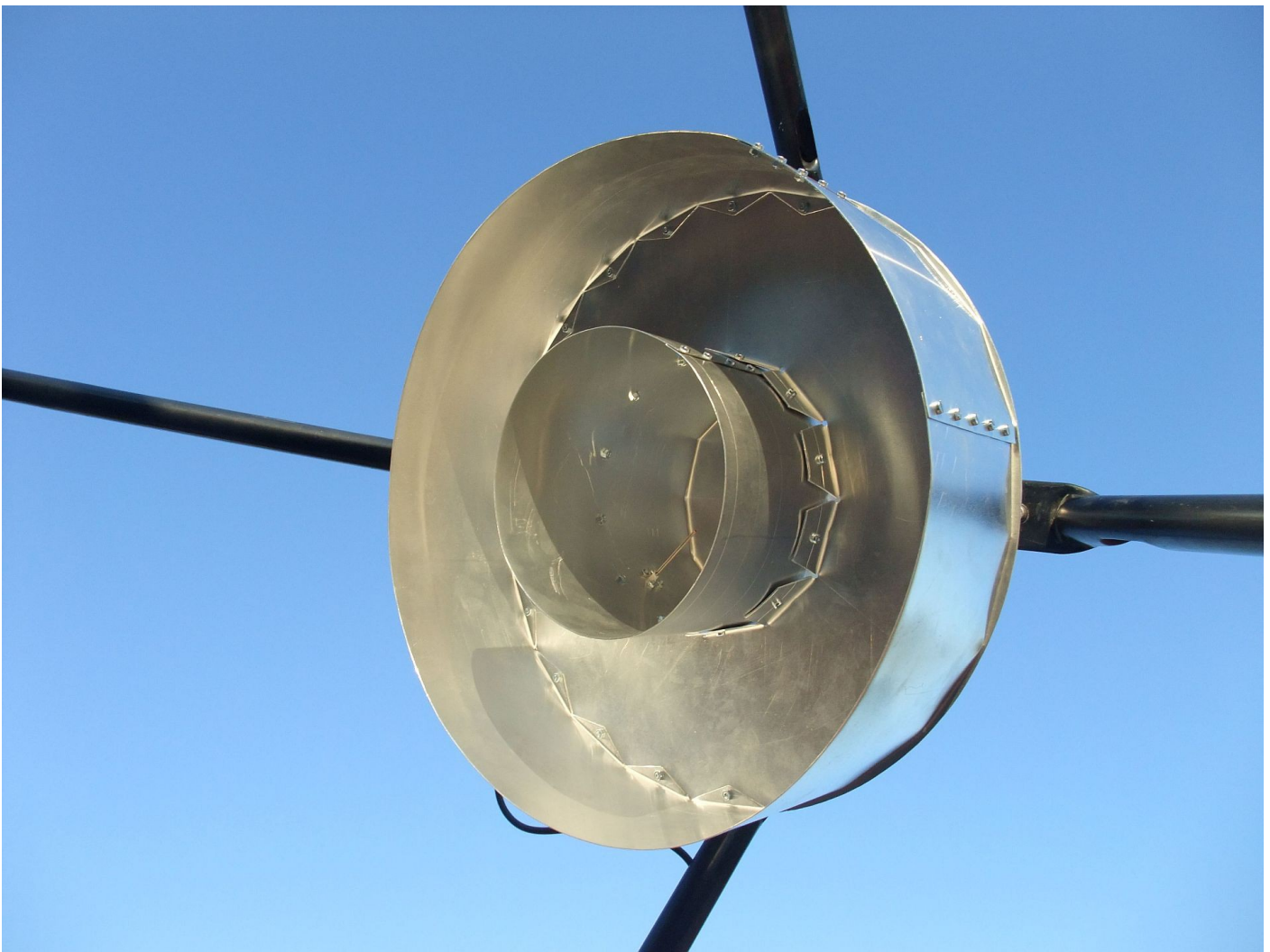
Figure 4: Practical implementation of the VE4MA feed.
