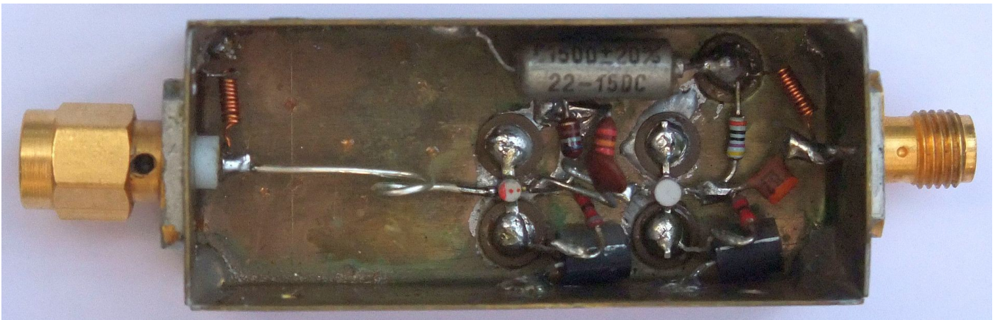
Figure 8: Practical implementation of the LNA.
