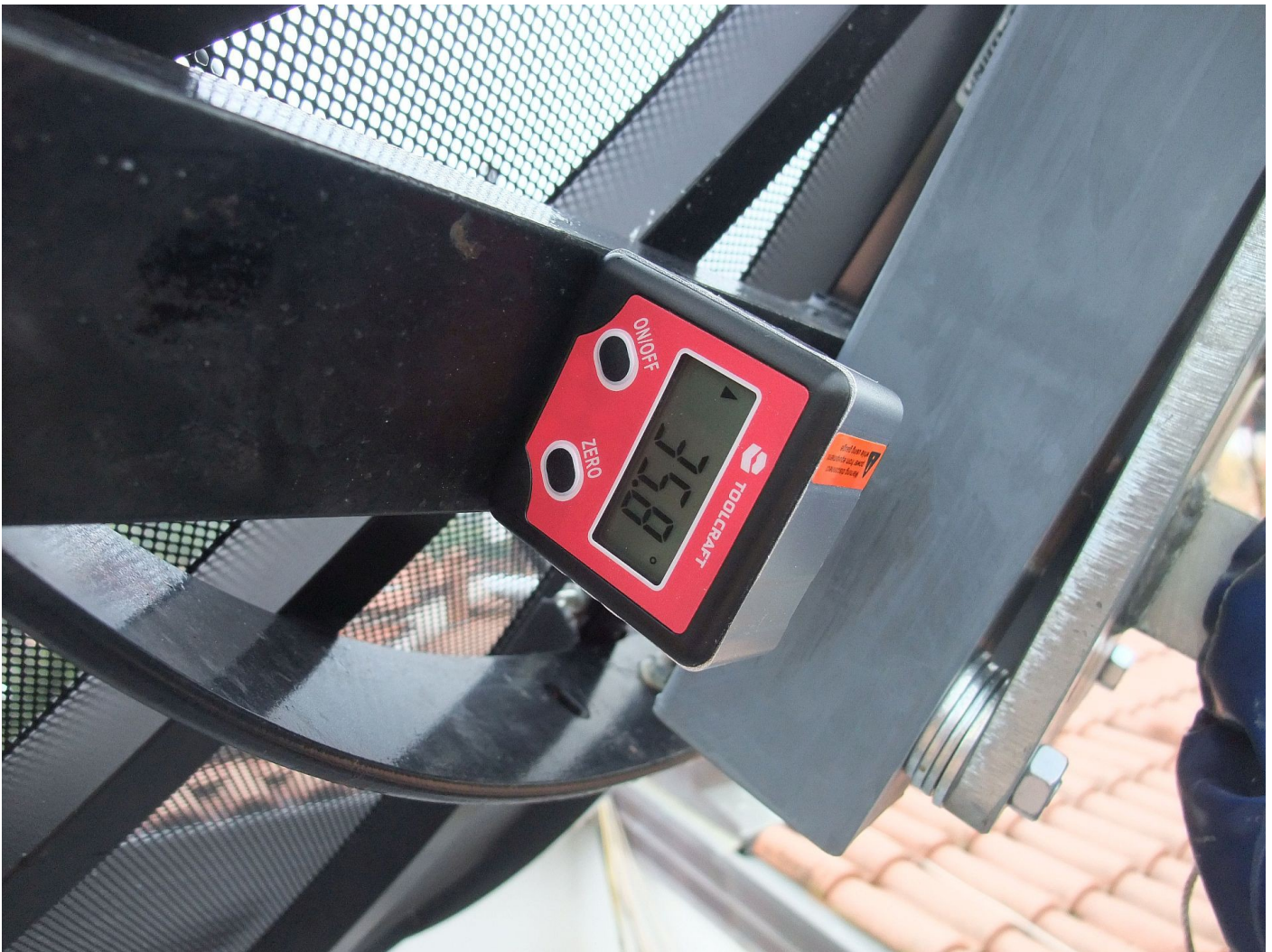
Figure 14: Using the inclinometer.
