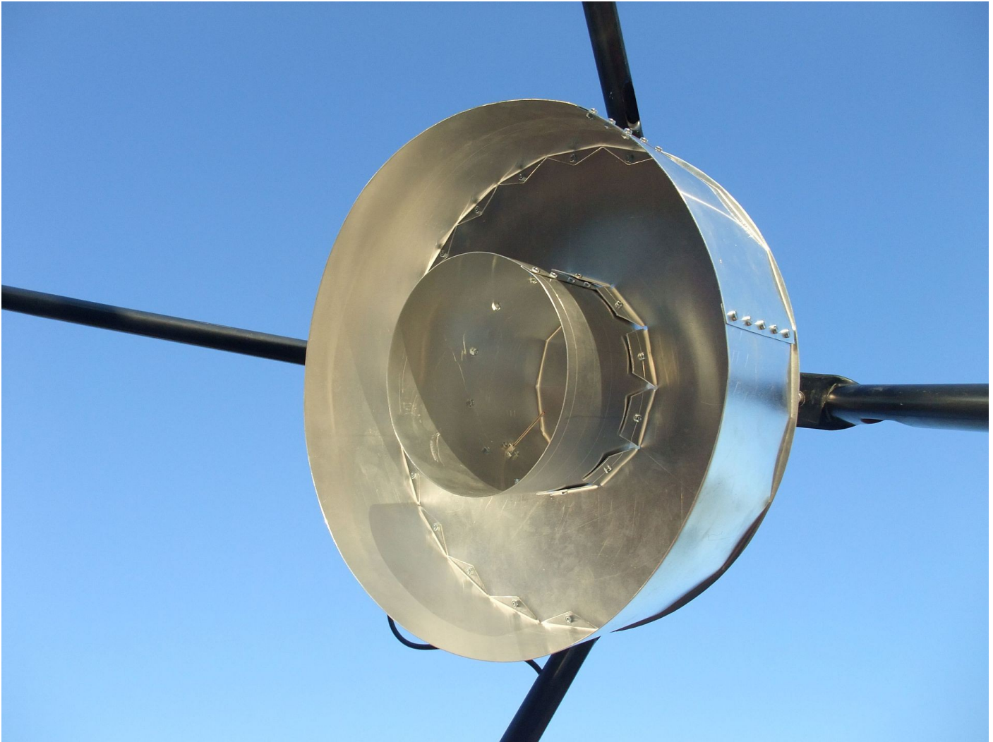
Figure 4: Practical implementation of the VE4MA feed.
