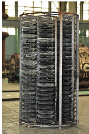
The growing chamber for quartz crystal
