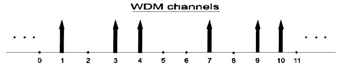
Fig. 3. TCC channel allocation obtained by repetition of three-channel islands, spaced k slots apart ( k = 2 in this example).
