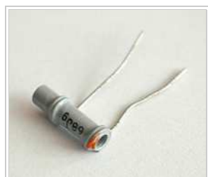
Ceramic tube capacitor, the typical style of ceramic capacitors in the 1950s and 1970s
