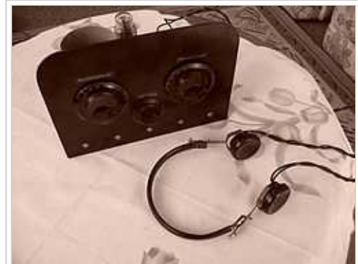
Homebuilt one-tube regenerative shortwave radio set with vintage headphones.
