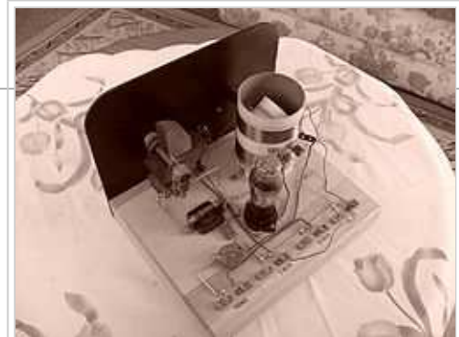
Rear view of the above radio, showing the simplicity of the regenerative design.
