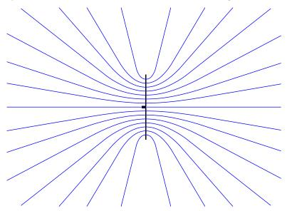
This figure indicates that the problem of a linear antenna can be regarded as a limiting case of a prolate spheroid, and that a solution might usefully be presented in prolate spheroidal coordinates [32].
